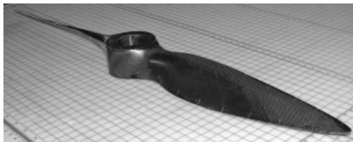
Compared to the props Hill regularly makes, there were some aspects of this prototype that required special treatment. The differences were mainly related to the thin tips of the prop. He knew that this was the optimal aerodynamic design for a race propeller. But one question lingered: would the thin tips hold?
