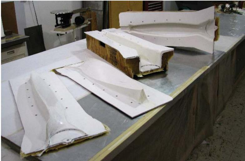
Steve Hill used the single blade prop master to make the four-piece mold shown above. When assembled, this mold was used to create the one-piece prototype propeller (right).
